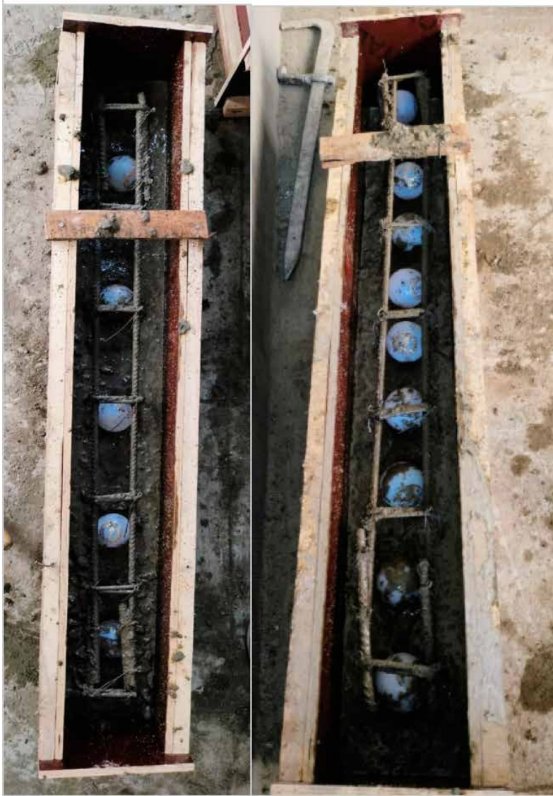
Figure.3 Placing of HDPE balls for different percentage of Volume reduction.
