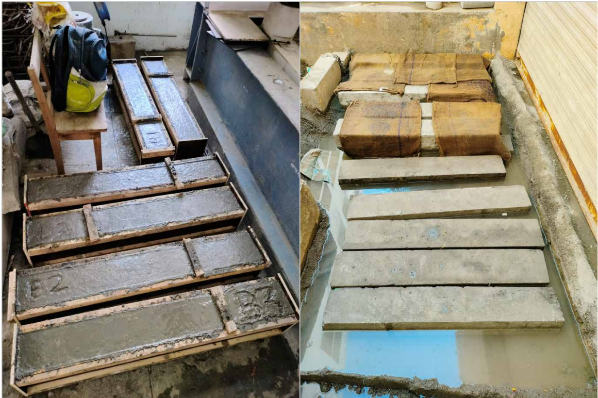
Figure.4 Casting and Curing of beam specimen.
