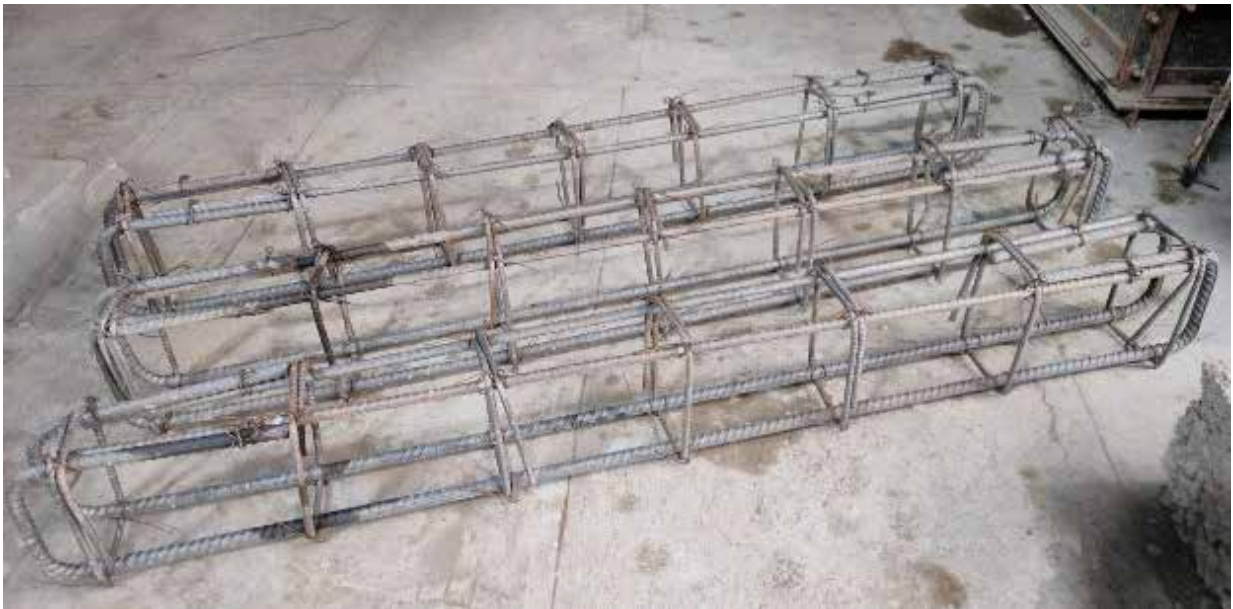
Figure.2. Reinforcement of beam specimen.
